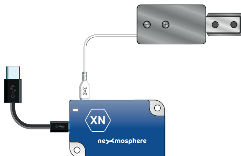
Example connection to XN Controller
